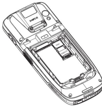
Figure 4-2 Insert the SIM Card
