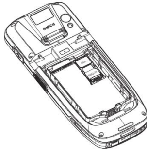
Figure 4-3 Place the SD Card in Card Slot
